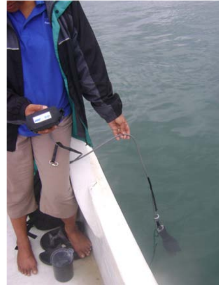
Measuring dissolved oxygen as a indicator of water quality of the Nadi basin.
