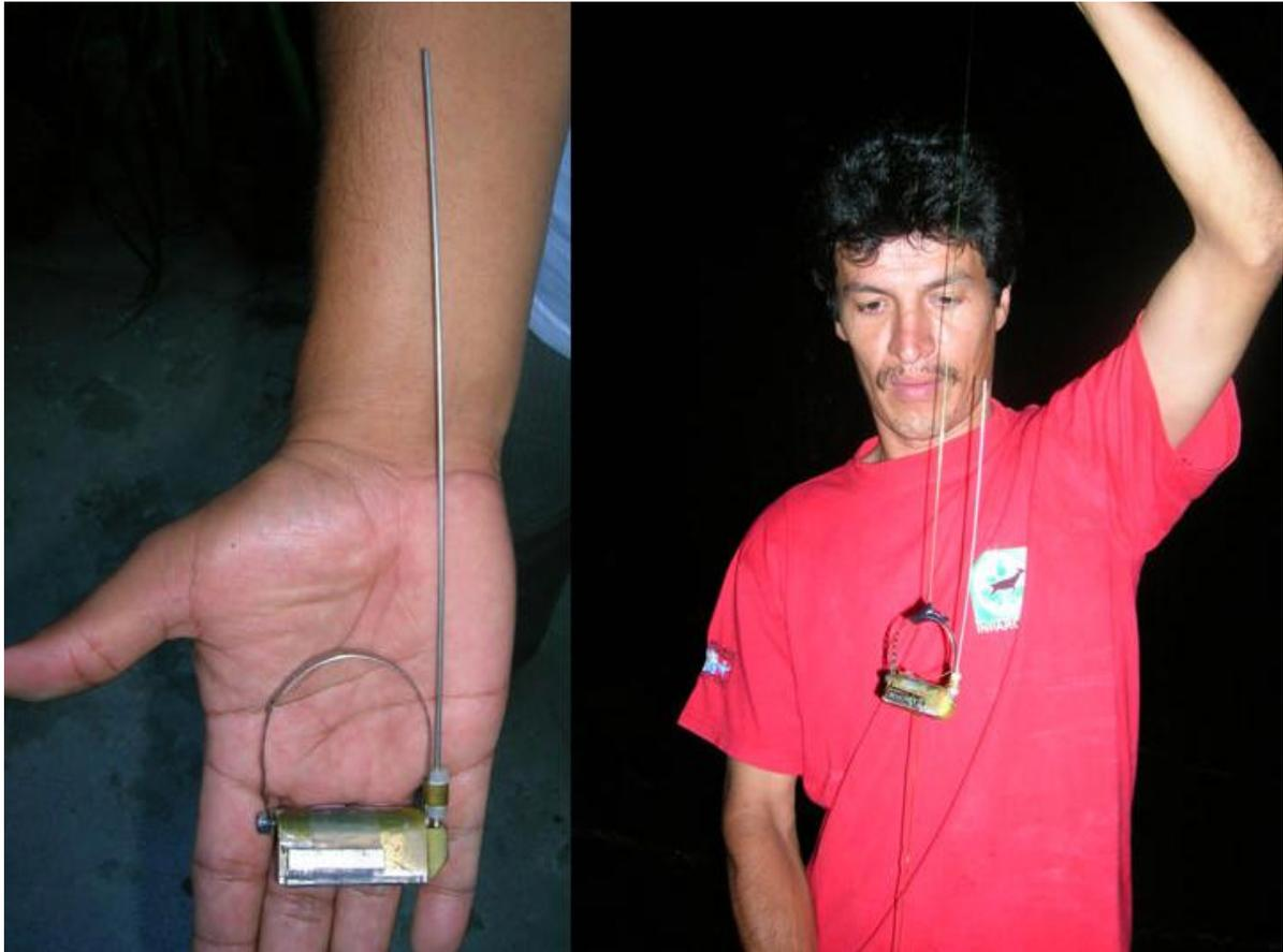
Figure 1: Satellite transmitter (PTT) designed and built for use on macaws by North Star Science and Technology
