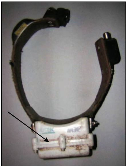
Photos 12-13. Left: “Shelved” battery case of the Lotek 3300SL GPS collar. Could this affect ice accumulation? Above: This collar collected ice over a four-day period. Interestingly it appears that the neck could not have fit in the collar with the iceball as seen in this photo made at recovery. The collar had been chewed. Could the chewing have resulted in additional ice accumulation?
