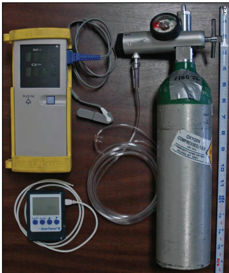
Photo 5. Pulse oximeter and continuous read thermometer along with the oxygen cylinder, regulator, and nasal cannula that are now integral components of our wolverine handling equipment. Total weight <7 lbs.
