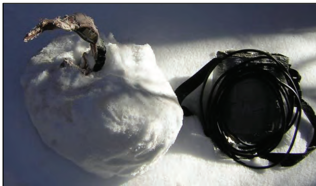
Photos 12-13. Left: “Shelved” battery case of the Lotek 3300SL GPS collar. Could this affect ice accumulation? Above: This collar collected ice over a four-day period. Interestingly it appears that the neck could not have fit in the collar with the iceball as seen in this photo made at recovery. The collar had been chewed. Could the chewing have resulted in additional ice accumulation?
